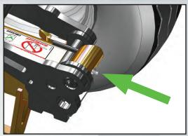
Always inspect for any evidence of physical damage such as bending, cracking, and any defects. If there is any damage, **DO NOT USE** and replace with an ITD cam lock.
