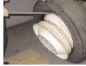
Stand assembly in vertical position with valve near top. Lubricate second bead and rim. Insert straight end of tool between tire bead and the back of the rim flange, hooking the tool over the top of the second flange. Lean tire assembly toward tool and provide a rocking or bouncing action to pry the rim out of the assembly.
