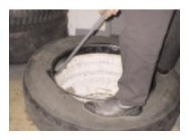
**Mounting:** Insert valve stem. Lubricate both bead seats of the rim and both tire beads. Push lower bead over flange and into rim well. Using curved end of tire iron with stop resting on rim flange, pry tire over flange, starting where tire bead crosses rim flange. Repeat progressively around tire working with small sections until the tire is completely over the rim.
