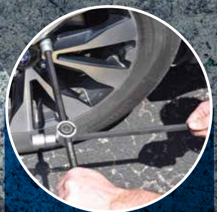
SLIDING ARMS GIVE EXTRA LEVERAGE FOR REMOVING LUG NUTS
