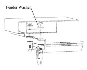
Inspect and retighten after first 10 uses
