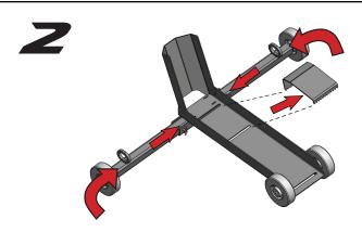
Install axles. Secure with pins. Remove ramp from storage slots.
