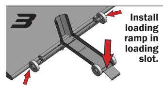
Ensure the Cycle Caddy is on level ground and positioned against the rear of the carrier deck before loading motorcycle
