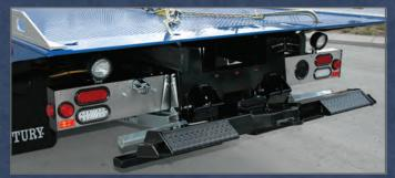
The low-profile fabricated wheel-lift stinger provides 68" of reach. When retracted, the crossbar is tucked in close to tailboard with minimal overhang. Century's 3-Way Pivoting L-arm System or the popular AutoGrip II crossbar are also available.
