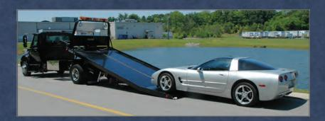
The Right Approach option available on Century 10 Series steel carriers eliminates the need for wood planks or ramps when loading and unloading low-clearance vehicles. The release handle allows the rear hinged deck section to be lowered to a 6-degree load angle. A removable cable guide is inserted in the deck to keep the cable low while winching the vehicle onto the rear deck.
