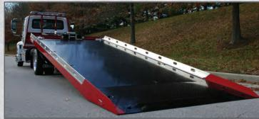
The innovative SST™ option provides a Solid Sloped Tail section that improves the load angle by 3 1/2 degrees.
