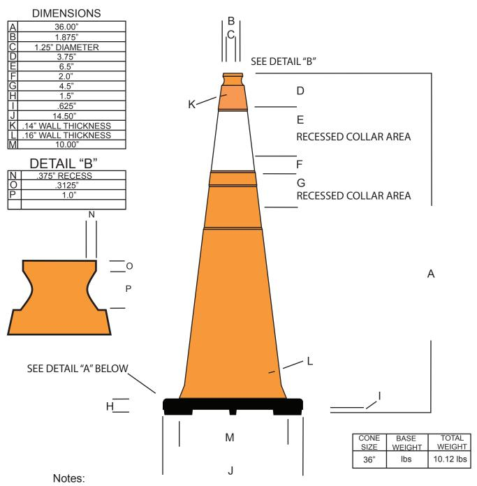
Conical section manufactured from 100% recyclable flourescent orange PVC Base manufactured form 100% post industrial recycled black PVC
