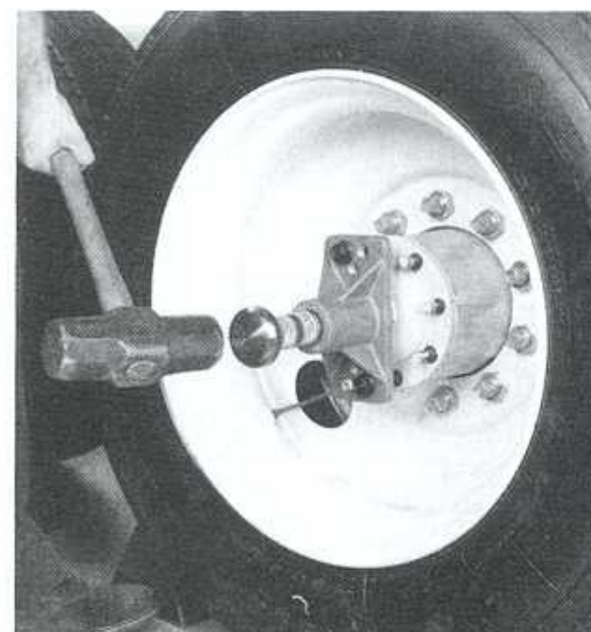
Drive Pin provides easy-to-hit target
