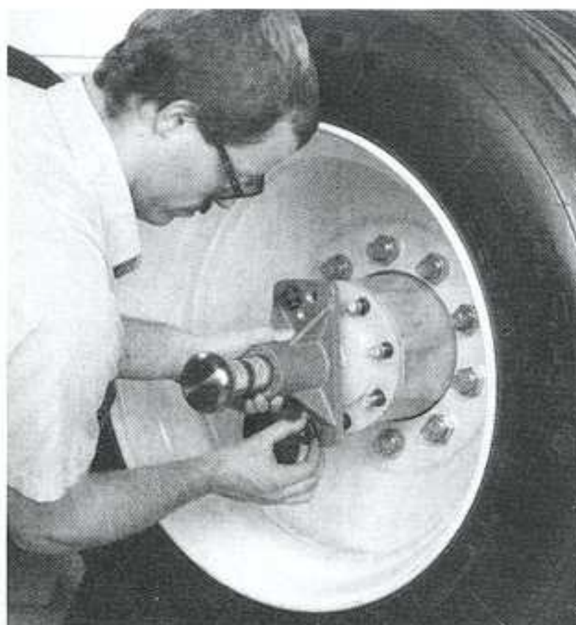
Install Drive Pin Plate Assembly
