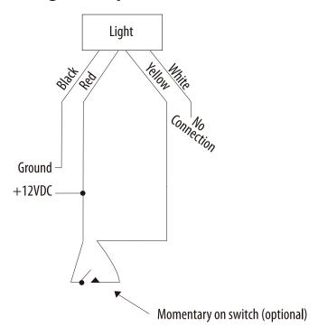
Make connections as in Steps 1 & 2. The white wire is not used for a single lamp installation.
