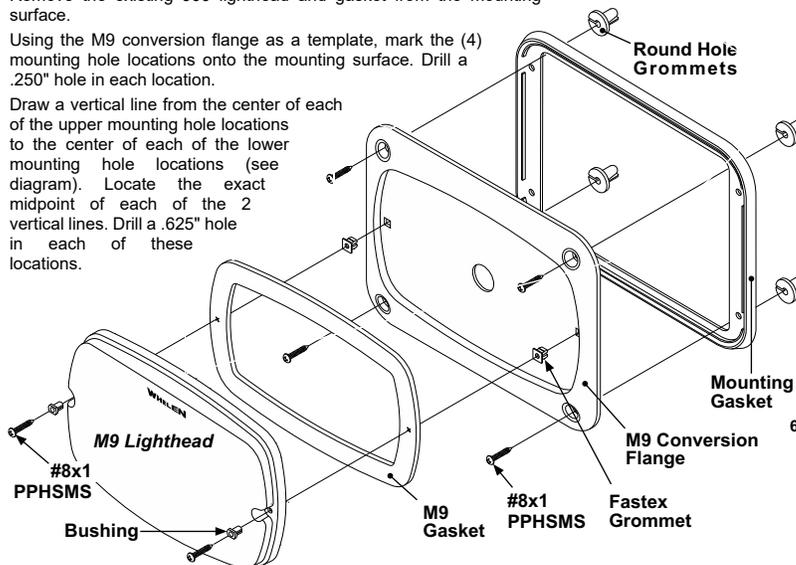
4. Assemble the bushing, lighthouse, gasket, Fastex grommets and conversion flange as shown. Insert the #8 x 1" screw as shown and tighten the assembly together.
