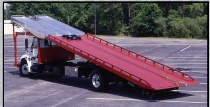
The deck over the cab tilts hydraulically for easy loading and unloading.
