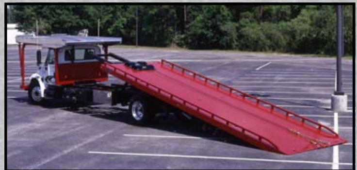
The deck over the cab tilts hydraulically for easy loading and unloading.
