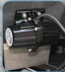
Prewired for Optional Vibrator Kit Shown Installed (3020340)
