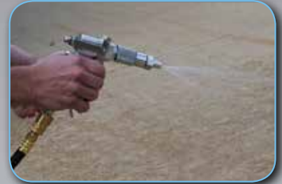
adjustable spray nozzle - pressure switch activates pump on demand
