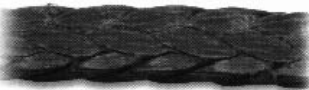
Rope exhibits fiber-set from compression. A slight sheen is visible. This is not a permanent characteristic and can be eliminated by flexing the rope.
