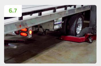
Confirm that the area around the truck is clear of any persons or obstructions. \*\*\*WARNING!\*\*\* During the synchronization process, all bed functions will operate while synchronizing.
