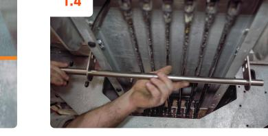
Install the two mounting tabs on each side of the crossover tunnel. Do not tighten completely. Place the actuator mounting bar through the mounting tabs so it aligns the two mounting tabs perpendicular and level to the control rods.
