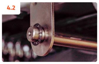
Install mounting bar retaining rings to each end of the actuator mounting bar.
