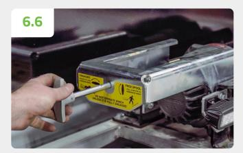
**IMPORTANT:** Shift the car carrier winch into free spool as it will activate during the synchronization process.
