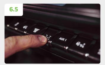
Engage the PTO. Activating the PTO provides power to the junction box.
