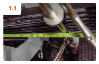
This remote system was designed to be attached to the crossover tunnel on the PASSENGER SIDE of the car carrier bed. A minimum of 17" length of space is required behind the control station hood for proper installation.
