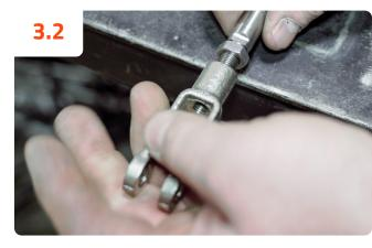
Thread the clevis onto the actuator pushrod. Make sure to thread the clevis up against the jam nut and torque the jam nut to 26 ft-lbs.
