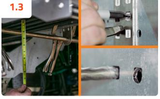
Allow for a 2" gap between the center of the actuator mounting bar below the car carrier control rods. Use the mounting tabs as a template to mark two drill points and drill two 7/16" holes on each side of the crossover tunnel.
