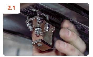
Loosely attach the C-bracket for each actuator to the designated control rod with the open end facing the actuator mounting bar.
