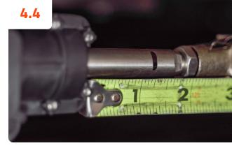
Confirm that the actuator pushrod is at or near an extension of 1-1/2".
