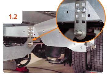
Install mounting tabs to the outside of the control rod crossover tunnel – close to the control station hood.
