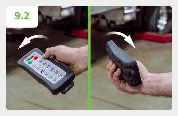
Rotate your wrist counter-clockwise to operate a function in the left column and the actuator will engage. The further the wrist is rotated, the further the control lever travels and the speed of the function will increase.
