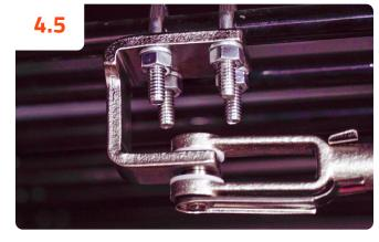
Insert the clevis pin into the clevis. To prevent corrosion, place one plastic washer on each side of the C-bracket, between the yoke of the clevis.
