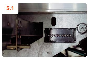
Locate a clear space on the side of the car carrier subframe past the end of the chassis frame. Install a junction box which provides a connection point for the 12V power supply from the PTO activating wire, a ground and 10 amp protected terminal(s) to connect to the actuators. **NOTE:** Actuators can be combined on a single ground or power terminal. The remote control system can also operate under a 24V system, if needed. A junction box is not provided with the SafeAll kit.
