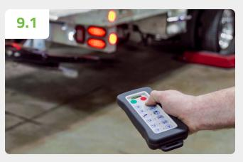
To engage the desired function, hold the remote in your hand in a horizontally and press and hold the button of the desired function.
