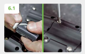
Remove the battery tray cover by removing the four cover screws from the remote. Install a 9V battery and reinstall cover.
