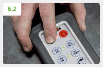
Press the green power button on the remote which will illuminate the red and green LEDs, confirming functionality. After two seconds, the green LEDs will display the battery power level. **NOTE:** The remote will automatically turn off after a three-minute period of inactivity.
