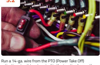
Run a 14-ga. wire from the PTO (Power Take Off) activation circuit to a terminal in the junction box so the actuators are live when the PTO is engaged.
