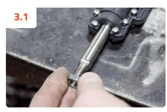
Thread the jam nut onto the actuator pushrod. Make sure to thread the jam nut all the way to the end of the threads.
