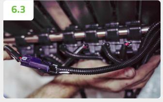
Only one actuator at a time can have power when synchronizing. **IMPORTANT:** Before synchronization a desired actuator function, the power source to all other actuators must be disconnected. Connect only one two-prong quick connector at a time when synchronizing.
