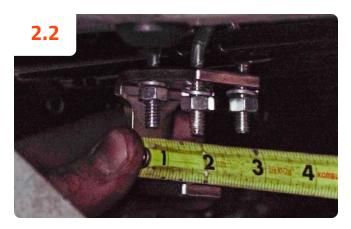
Measure 16-3/4" from the center of the actuator mounting bar to the back side of the C-bracket. Ensure the C-bracket is positioned vertically so the actuator is parallel to the control rods. Tighten the U-bolt nuts evenly and torque to 5 ft-lbs. \*\*\*WARNING!\*\*\* The C-brackets must be secured tightly. Loose C-brackets WILL result in system failure!
