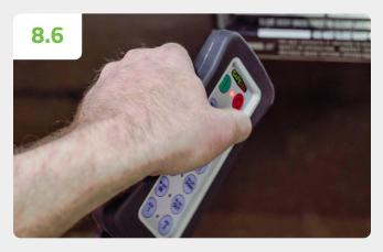
Press and release the RIGHT button of desired function. The remote will then engage the powered actuator until it reaches the maximum travel. **NOTE:** Watch the corresponding control lever on the car carrier and verify maximum travel.
