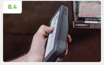
Press and release the LEFT button of desired function. The remote will then engage the powered actuator until it reaches the maximum travel. **NOTE:** Watch the corresponding control lever on the car carrier and verify maximum travel.
