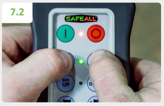
Hold both right and left buttons in the desired row for a period of 10 seconds. Once 10 seconds has elapsed, the green LED will turn off; then release the buttons.
