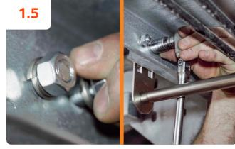
Install carriage bolts, lock washers and nuts to complete the connection of the mounting tabs to the crossover tunnel. Torque each nut to 30ft-lbs. \*\*\*WARNING!\*\*\*
