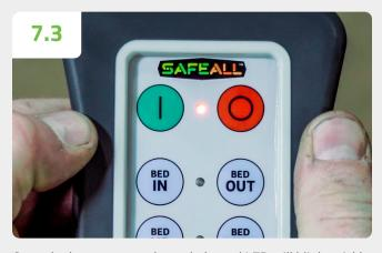
Once the buttons are released, the red LED will blink quickly. This indicates the remote is searching for the powered actuator. Once the handheld finds the actuator, the red LED will blink slowly, which indicates synchronization is in process. When the green LED illuminates a steady light, the synchronization is complete. **NOTE:** If the green LED does not illuminate, repeat Step 7.2.
