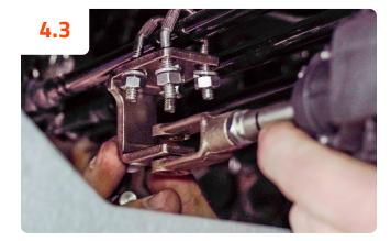
Manually pull or push the actuator pushrod into position so the clevis aligns with the C-bracket hole.
