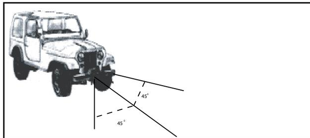
Winches equipped with cable guide fairleads can pull from several directions. Pull from an angle only to straighten out the vehicle—otherwise you can damage structural members or other parts of your vehicle and cause excess cable buildup on one end of the winch drum.
