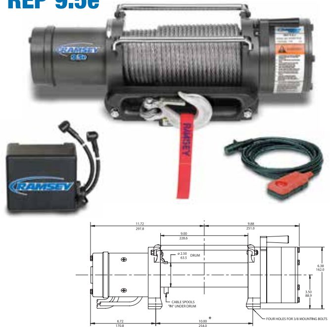
* MOUNTING BOLT PATTERN: FOUR 4-HI HOLES IN A 10.00±.015 x 4.50±.015 (254.0mm x 114.3mm) RECTANGULAR PATTERN
