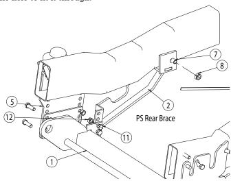
**6.** Position the DS Rear Brace (3) to the frame and secure it onto the Pushbar (1) with two ½-13 fasteners (11 & 12). Look to the back of the Rear Brace (3), and temporarily install the U-bolt (9) onto the frame. Mark and drill the two holes Ø.531" through one wall. Undo the U-bolts and insert the bolt-sticks (6) through the newly drilled holes. Finally, re-insert the U-bolt and secure the Rear Brace (3) to the truck-frame with proper nuts and a spacer (10).
