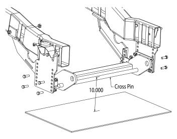
**5.** Position the PS Rear Brace (2) to the frame and secure it onto the Pushbar (1) with two  $\frac{1}{2}$ -13 fasteners (11 & 12). In the back, secure the Rear Brace to the truck-frame using one  $\frac{5}{8}$ -11 x 5 bolt (7) and one  $\frac{5}{8}$ " nuts (8). You may have to enlarge the hole to fit it through.
