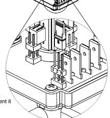
6. <u>SHORTCUTS</u>: Use the "shortcuts" shown in the chart below to make the programming of your light easier: Hold the green wire to ground (or hold the Pattern Select Button or hold the Jumper to Pins 1 & 2) for the indicated amount of time to go directly to the indicated pattern.
