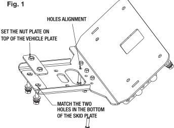
**3.** Align Driver Rear Brace Stiffener (3) plate onto the Skid Plate (1). Secure it with two 3/8 bolts (11, 12) & two 3/8 lock nuts (10).
