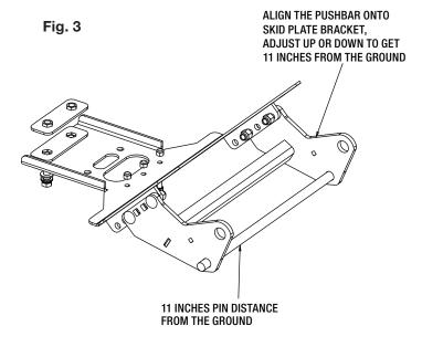
6. Torque all fasteners as shown in the chart. Check and re-torque all fasteners after 5 hours of usage to ensure safe plow operation.
