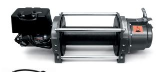
The Series 9 DC features a weatherproof industrial contactor and heavy duty remote control. The disc brake is designed for extended power-out use and the motor is protected by a thermal over-load switch. Its lower gear ratio of 199:1 provides a fast line speed. Designed to meet SAE J706 and CE standards.
