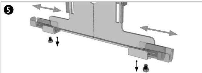
Unscrew the screws at the bottom sides of the holder to adjust the tablet holder's width to the tablet. Tighten to secure.
