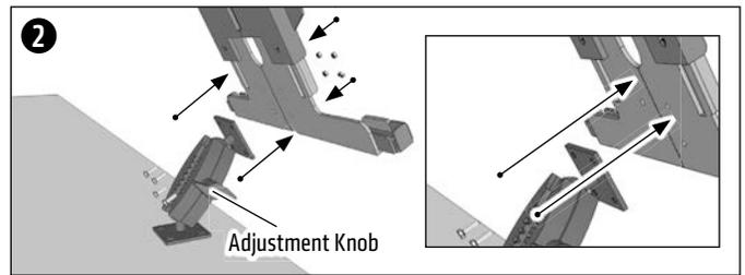
Connect the tablet holder to the mounting base (screws provided) using the 4-Hole AMPS mounting pattern. Loosen adjustment knob to reposition shaft, retighten to desired position.
