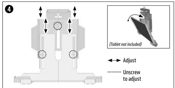
Unscrew the three screws/washers at the back/center of the holder to adjust the tablet holder's height to the tablet (not included). Retighten the screws/washers to secure.
