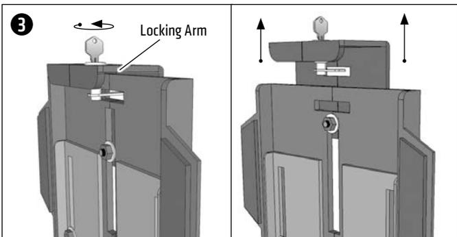
To size the tablet holder to your tablet, begin by unlocking the top of the tablet holder with the key and push up on the locking arm.
