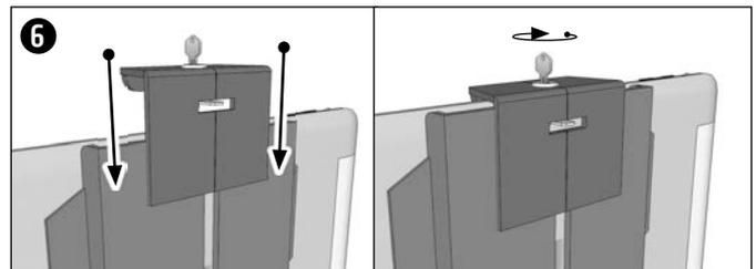
To lock down tablet, close down on the locking arm on the top of the tablet and lock with key (included).
