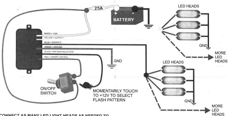
CONNECT AS MANY LED LIGHT HEADS AS NEEDED TO EACH OF THE OUTPUT WIRES. DO NOT EXCEED THE MAXIMUM CURRENT RATING OF THE OUTPUT WIRES (10A).
