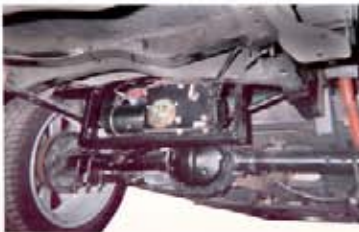
Oasis Air Compressor mounted under truck.
